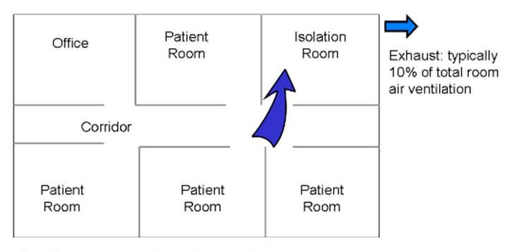
Specific areas should be under negative pressure to prevent cross contamination to other areas of the building (0.001" W.G. or 100 FPM inward velocity)
